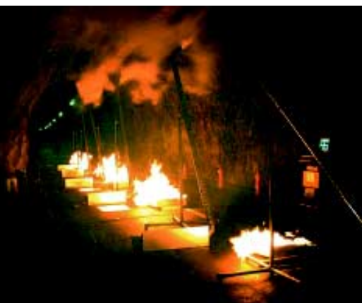
Hot smoke test in a tunnel
