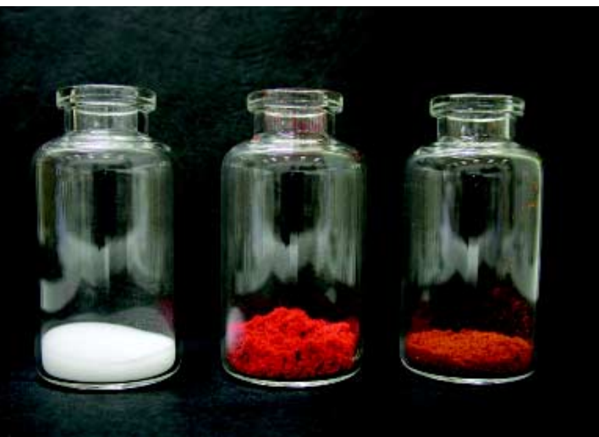
Silica gel as support (white) impregnated with red pigment yields the end product (right)
