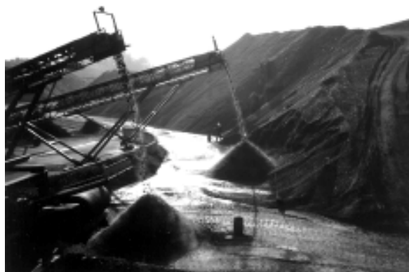
Conventional aging and treatment of bottom ashes from thermal waste incineration plants
