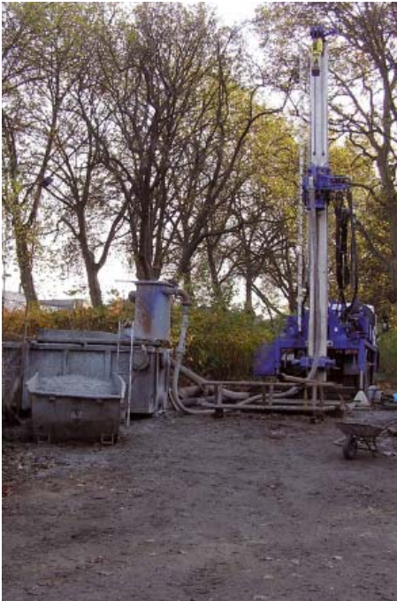
View of an exploratory drilling at the former Dorstfeld mine in Dortmund. Here coal mine gas is extracted night and day.
